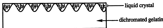
Figure 6. Liquid-crystal-filled relief grating. When a holographic grating is recorded in dichromated gelatin, a surface relief structure is obtained, because of shrinkage in the exposed regions. By filling the grooves with a nematic liquid crystal and sandwiching between transparent electrodes, a switchable hologram is obtained.
