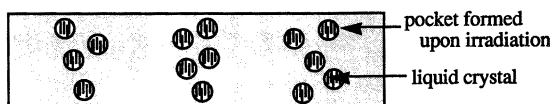
Figure 7. Liquid-crystal-filled DMP-128 photopolymer. Upon holographic irradiation, Polaroid's DMP-128 forms air pockets in the light regions. When these pockets are filled with a nematic liquid crystal, a switchable hologram results.
